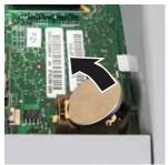
Carefully pry with screwdriver here
